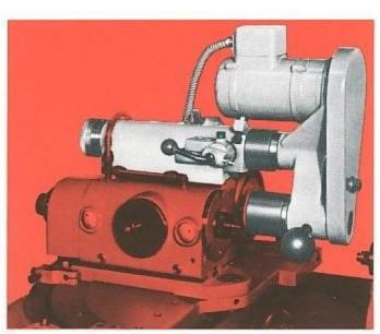
Face grinding device to square a face to a ground bore.
